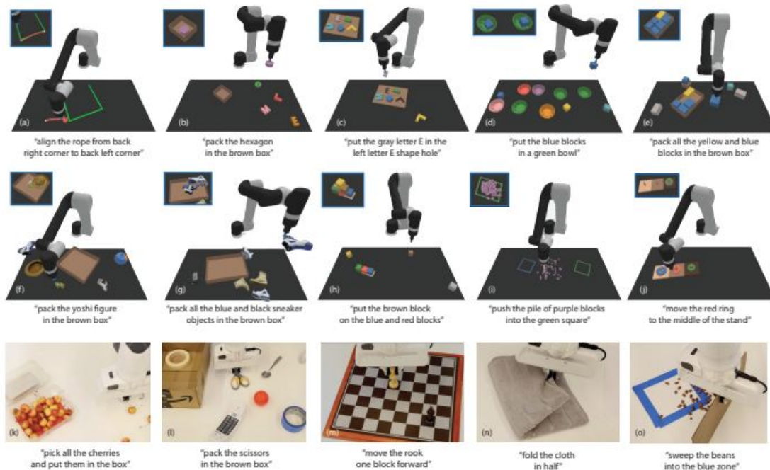
Figure 1. Language-Conditioned Manipulation Tasks: CLIPORT is a broad framework applicable to a wide range of language-conditioned manipulation tasks in tabletop settings. We conduct large-scale experiments in Ravens [2] on 10 simulated tasks (a-j) with 1000s of unique instances per task. See Appendix A for challenges pertaining to each task. CLIPORT can even learn one multi-task model for all 10 tasks that achieves better or comparable performance to single-task models. Similarly, we demonstrate our approach on a Franka Panda manipulator with one multi-task model for 9 real-world tasks (k-o; only 5 shown) trained with just 179 image-action pairs.
