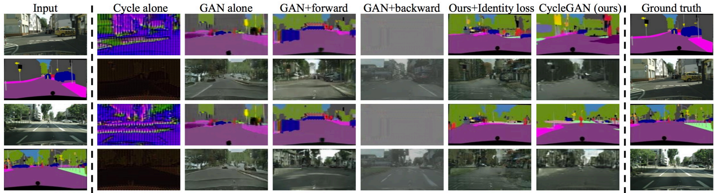
Figure 7: Different variants of our method for mapping labels \leftrightarrow photos trained on cityscapes. From left to right: input, cycle-consistency loss alone, adversarial loss alone, GAN + forward cycle-consistency loss ( F(G(x)) \approx x ), GAN + backward cycle-consistency loss ( G(F(y)) \approx y ), CycleGAN (our full method), and ground truth. Both Cycle alone and GAN + backward fail to produce images similar to the target domain. GAN alone and GAN + forward suffer from mode collapse, producing identical label maps regardless of the input photo.
